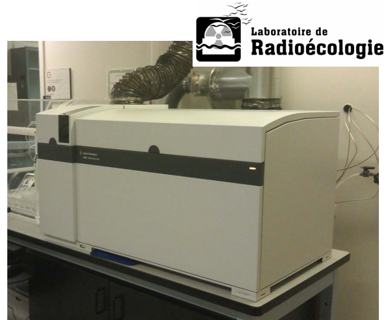
ICP-MS: Agilent 8800 QQQ (Agilent) Liquid chromatography (Dionex/ThermoFisher) Autosampler (ThermoFisher)
