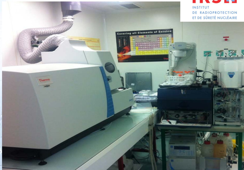
ICP-MS: X-SERIES II (ThermoFisher) Liquid chromatography (Dionex/ThermoFisher) Autosampler (ThermoFisher)
